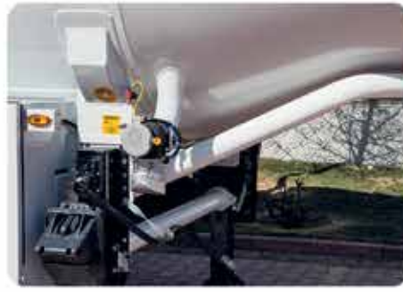
Vapour recovery adaptor, ground connection, emergency stop, wheel chock Buhar geri dönüşüm adaptörü, Topraklama, Acil stop butonu, teker takozu
