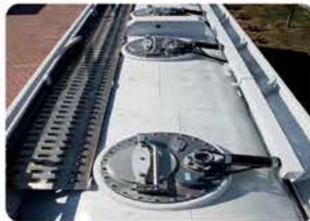
DN500 loading manhole covers with vapour recovery valve, overfill protection system DN500 dolum kapağı, buhar tahliye ventili, taşma önleyici sistem
