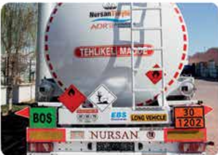
Aluminium ladder, Aluminium rear bumper, ADR lighting system, EBS / ABS Alüminyum merdiven, Alüminyum tampon, ADR aydınlatma sistemi, EBS / ABS
